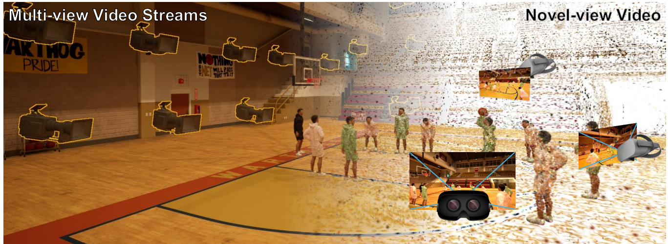
Fig. 1. LiveSplats takes multi-view video streams of sports events as input and reconstructs the dynamic 3D scene to allow viewers to watch from any novel view with interactive frame rates.
