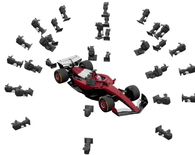
Fig. 1: Hemispherical initialization rig. At t = 0 , a dense hemisphere of cameras surrounds each vehicle to bootstrap a high-quality first-frame Gaussian reconstruction. This provides the initial 3D representation that streaming methods then propagate forward in time. Hemisphere views are used only for initialization and are excluded from all evaluation metrics.
